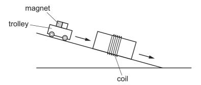
An electromotive force (e.m.f.) is induced in the coil. A graph of the e.m.f. against time is plotted.
